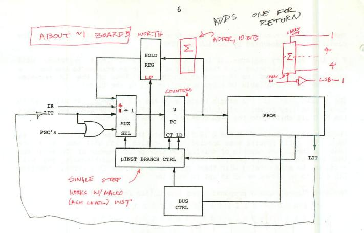
The CPU will probably not fit on a single board. Partitioning it between two boards will be a major headache due to the very limited number of unused pins on the edge connectors. Think about this one carefully!
