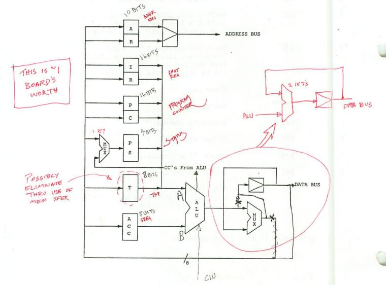
The PS register can be loaded either from the URCPU internal bus or from the condition bits generated by the ALU and URMP.
