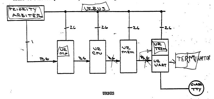
NOTE: Since we will be using a wired-OR feature of the CMOS Open Drain 74C906 parts to deal with the major bus control signals, it is advantageous to use low signal levels to indicate a particular action (i.e. negative logic). In order to be compatible with the handout we will adopt a negative logic
